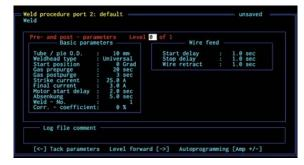
Obviously the ORBIMAT 165 CBasic includes the well proven ORBIMATIC AUTOPROGRAMMING with easy weld procedure generation, with requires input of Diameter, Wall thickness, Material and Gas, as well as the current slope function between a maximum 99 different Welding Levels. The standard version of the ORBIMAT 165 CBasic includes the control system for cold-wire-feeding and is therefore able to run the complete range of ORBIMATIC Weld heads.
